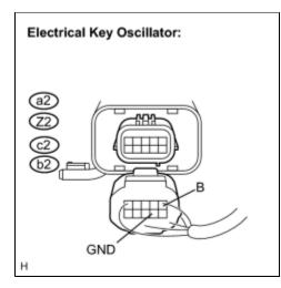
(a) Disconnect the oscillator connectors.
