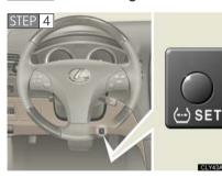
Press the tire pressure warning reset button for more than 3 seconds. At this time, the tire inflation pressure warning indicator flashes 3 times.
