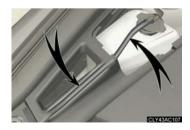
When installing the reservoir cap, make sure that the engine coolant reservoir hose positioned as shown in the illustration.
