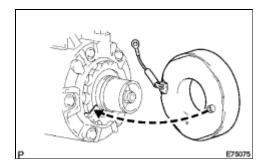
(a) Install the magnetic clutch stator while aligning the protrusion on the stator with the notch on the air compressor assembly as shown in the illustration.
