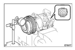
(a) Set the dial indicator to the magnetic clutch hub.
