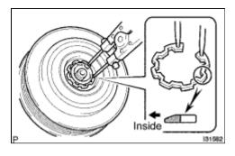
(d) Using a snap ring expander, install the magnetic clutch rotor and a new snap ring with the chamfered side facing up.
