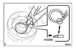
(b) Using a snap ring expander, install a new snap ring with the chamfered side facing up.
