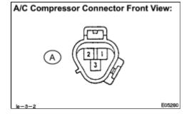
(a) Disconnect the connector from the compressor and magnetic clutch.
