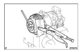
(a) Place the compressor and magnetic clutch in a vise.
