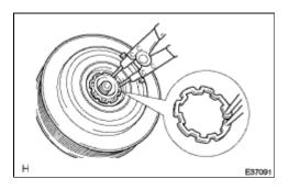
(d) Using a snap ring expander, remove the snap ring and then remove the magnetic clutch rotor.
