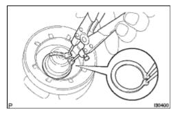
(g) Using a snap ring expander, remove the snap ring and magnetic clutch stator.
