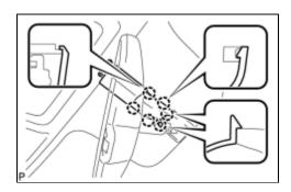
(b) Disengage the 6 claws and remove the inner rear view mirror stay holder cover.
