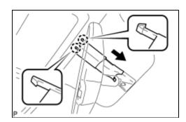
(a) Disengage the 2 claws and slide the inner rear view mirror stay holder cover as shown in the illustration.
