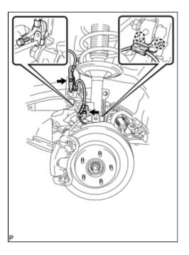
(b) Remove the 2 bolts from the body and the shock absorber assembly.
