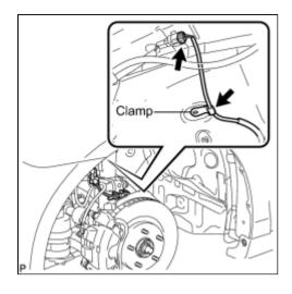
(a) Disconnect the front speed sensor connector and clamp.
