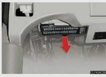
▶ Driver's side instrument panelRemove the lid.
