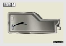
Remove the fuse with the pullout tool.
