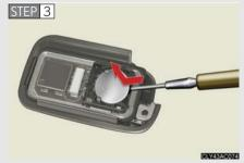
Remove the depleted battery.
