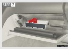
Open the glove box. Remove the glove box cover.
