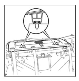
(b) Pass the 3 rear seat belt floor anchors through the holes in the package tray trim panel assembly.
