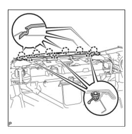
(a) Disengage the 3 clips and 6 claws, and remove the No. 2 package tray trim panel assembly.
