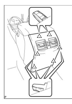
(a) Engage the 6 clips and install the console rear end panel sub-assembly.
