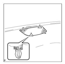
(a) Engage the 4 clips and install the No. 1 speaker hole cover.
