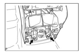
(e) Install the rear console box assembly with the 2 bolts <E>.
