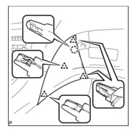
(a) Engage the claw and 4 clips to install the instrument panel finish panel end RH.
