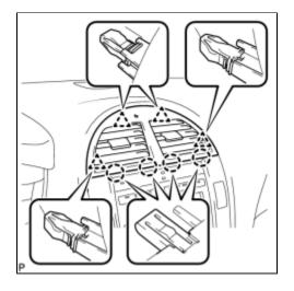
(b) Engage the 4 claws and 4 clips, and install the No. 2 instrument panel register assembly.
