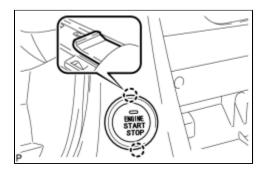
(b) Engage the 2 claws and install the push start switch.
