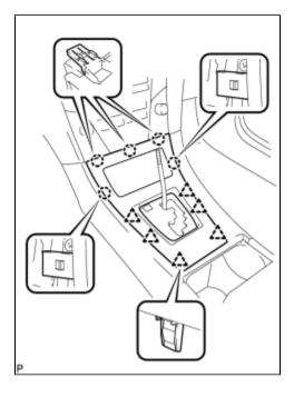
(b) Engage the 5 claws and 6 clips to install the upper console panel assembly with front ash receptacle.
