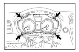
(b) Install the combination meter assembly with the 4 screws  $\langle B \rangle$  or  $\langle C \rangle$ .
