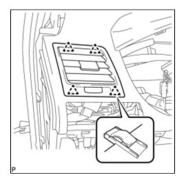
(a) Engage the 4 clips and install the No. 1 instrument panel register assembly.
