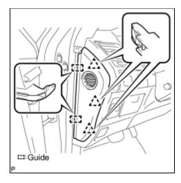
(c) Engage the 2 guides and the 3 clips to install the side instrument panel LH.
