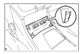
(b) Engage the 4 clips and install the heater seat switch base.
