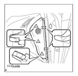
(c) Engage the 2 guides and the 3 clips to install the side instrument panel RH.
