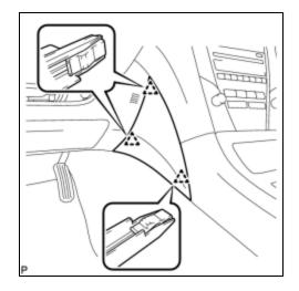
(a) Engage the 3 clips and install the instrument panel finish panel end LH.
