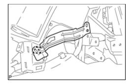
(a) Install the clip and the No. 1 instrument panel mounting bracket.
