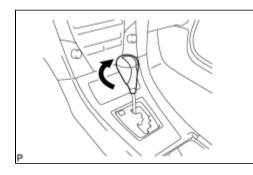
(a) Install the shift lever knob sub-assembly.
