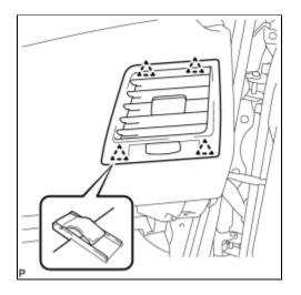
(a) Engage the 4 clips and install the No. 3 instrument panel register assembly.
