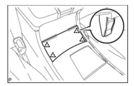
(a) Engage the 4 clips and install the heater seat switch base.
