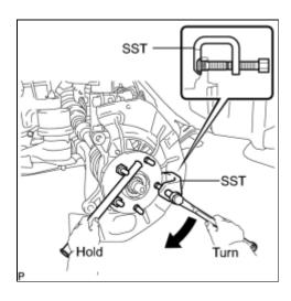
(a) Temporarily install the 2 nuts and washers to the front axle hub bolt as shown in the illustration.
