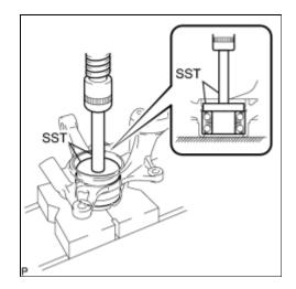
(a) Using SST and a press, install a new front axle hub bearing to the steering knuckle.
