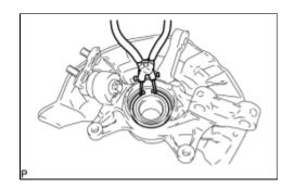
(a) Using snap ring pliers, install a new front axle hub hole snap ring.
