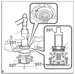
(a) Using SST and a hammer, install a new No. 1 front wheel bearing dust deflector.
