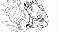
(a) Install the front disc brake caliper assembly to the steering knuckle with the 2 bolts.
