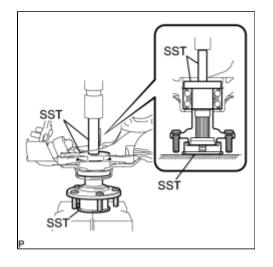
(a) Using SST and a press, install the front axle hub sub-assembly.
