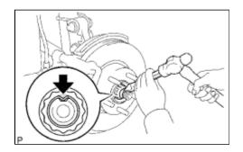
(a) Using a chisel and hammer, stake the axle hub nut.
