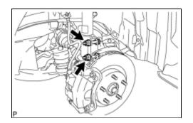
(b) Install the steering knuckle with the front axle assembly to the front shock absorber with the 2 bolts and 2 nuts.
