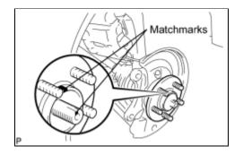
(a) Align the matchmarks and install the front drive shaft assembly to the front axle hub sub-assembly.
