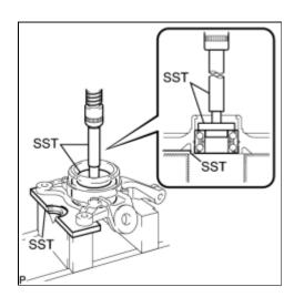
(c) Using SST, support the steering knuckle horizontally. Place it on the V-blocks as shown in the illustration.
