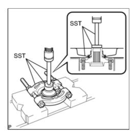
(c) Using SST and a press, remove the bearing inner race (outside) from the front axle hub sub-assembly.
