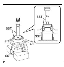
(b) Using SST and a press, press the front axle hub bearing until it contacts the SST.
