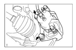
(a) Remove the 2 bolts and separate the front disc brake caliper assembly from the steering knuckle.
