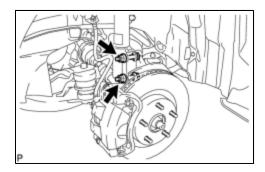
(c) Remove the 2 bolts, 2 nuts, and front axle assembly.
