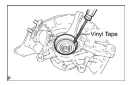
(a) Using a screwdriver with its tip wrapped with vinyl tape, remove the No. 1 front wheel bearing dust deflector.
