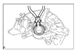
(a) Using snap ring pliers, remove the front axle hub hole snap ring.
