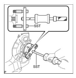
(b) Using SST, remove the front axle hub sub-assembly.
