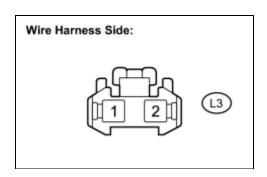
(a) Disconnect the high mounted stop light connector.
