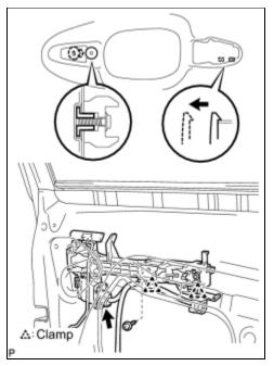
(a) Using a "TORX" socket wrench (T30), loosen the screw.
