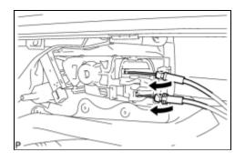
(f) Disconnect the cables and each connector from the back side of the inside handle and remove the front door trim board sub-assembly.
