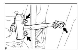
(a) Remove the bolt, 2 nuts, and front door check assembly.
