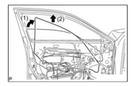
(b) Remove the front door glass sub-assembly as shown in the illustration.
