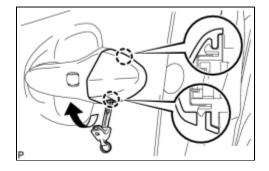
(a) Using an emergency key, disengage the 2 claws and remove the front door outside handle cover.
