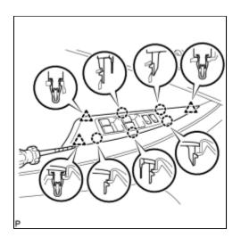
(a) Using a screwdriver with the tip wrapped with protective tape, disengage the 5 claws and 3 clips, and remove the front door armrest base panel assembly.
