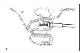
(b) Remove the front door inside locking cable assembly.
