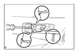
(a) Using a screwdriver with the tip wrapped with protective tape, disengage the 3 claws, and remove the front door inside handle bezel plug.
