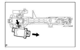
(a) Remove the screw and door electrical key oscillator.
