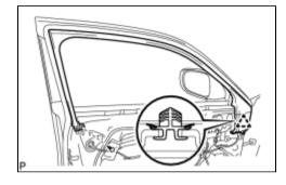
(a) Using a clip remover, remove the clip.
