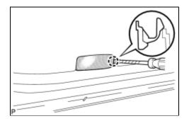
(a) Using a screwdriver with the tip wrapped with protective tape, disengage the claw and remove the courtesy light assembly.
