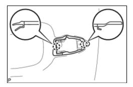
(a) Disengage the 2 claws and remove the front door rear outside handle pad.
