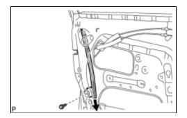
(a) Remove the bolt and the front door rear lower frame sub-assembly as shown in the illustration.
