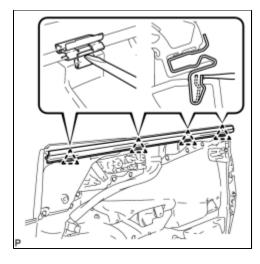
(a) Disengage the 4 clips as shown in the illustration and remove the front door inner glass weatherstrip from the front door trim board.
