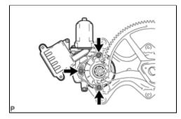
(a) Using a "TORX" driver (T25), remove the 3 screws and the front power window regulator motor assembly.
