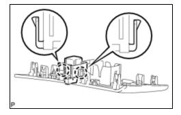
(a) Disengage the 2 claws and remove the door control switch assembly.
