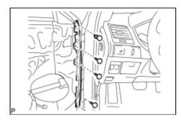
(a) Using a clip remover, disengage the 4 clips and remove the front No. 3 door weatherstrip.
