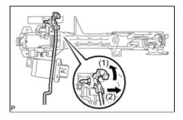
(a) Remove the front door lock open rod as shown in the illustration.
