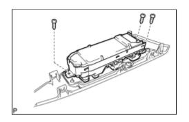
(a) Remove the 3 screws and the power window regulator master switch assembly.
