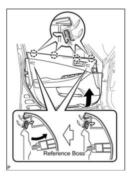
(c) Pull up the front door trim board in the direction indicated by the arrow.
