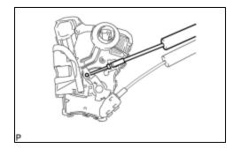
(a) Remove the front door lock remote control cable assembly.
