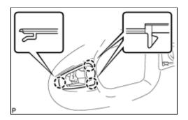
(a) Disengage the 3 claws and remove the front door front outside handle pad.
