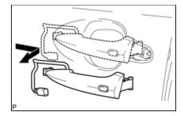
(e) Remove the front door outside handle assembly as shown in the illustration.
