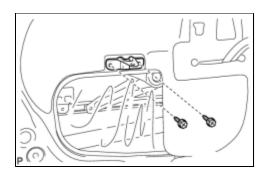
(a) Remove the 2 screws and the front No. 1 door trim bracket.
