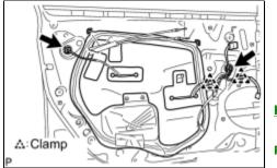
(a) Disconnect each connector and each clamp, and remove the front door service hole cover.
