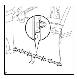
(a) Using a moulding remover, disengage the 7 clips.
