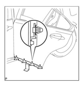
(a) Using a moulding remover, disengage the 4 clips.
