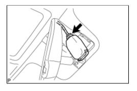
(b) Disconnect the connector and remove the rain sensor.
