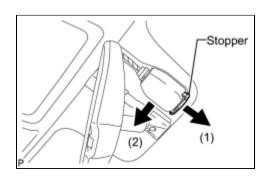
(a) Release the stopper by pulling the stopper down and disconnect the rain sensor as shown in the illustration.
