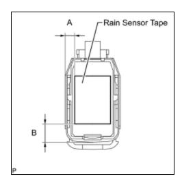
(a) Remove the releasing sheet (yellow side) from new rain sensor tape and apply the tape to the position indicated in the illustration (the sensor part of the rain sensor) while pushing out air bubbles with your fingers.
