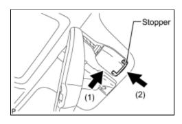
(b) Gradually attach the rain sensor to the glass surface to prevent air bubbles from forming between them.
