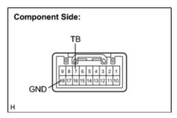
(a) Measure the resistance according to the value(s) in the table below. Standard resistance:
