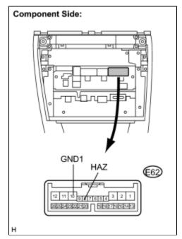
(a) Measure the resistance according to the value(s) in the table below. Standard resistance:
