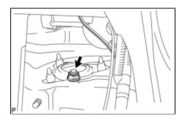
(e) Fully tighten the lock nut.
