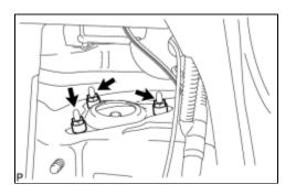
(c) Install the 3 nuts to the upper side of the rear shock absorber with coil spring.
