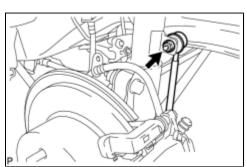
(a) Install the rear stabilizer link assembly LH to the rear shock absorber with the nut.
