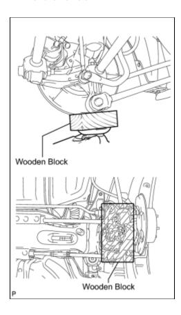
(b) Slowly jack up the vehicle using a wooden block and install the rear shock absorber with coil spring (upper side) to the vehicle.
