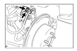
(a) Install the rear brake flexible hose and rear speed sensor wire harness with the 2 bolts.
