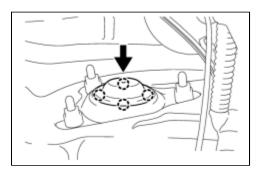
(a) Engage the 4 claws and install the rear suspension support No. 1 cover.
