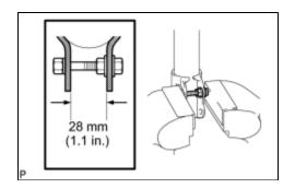
(a) As shown in the illustration, secure the rear shock absorber with coil spring in a vise using aluminum plates by closing the vise onto the double nutted bolt affixed to the bracket at the bottom of the absorber.
