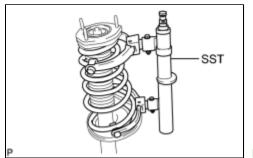
(a) Using SST, compress the rear coil spring.
