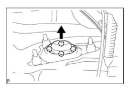
(a) Remove the 4 claws and the rear suspension support No. 1 cover.
