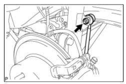
(a) Remove the nut and separate the rear stabilizer link assembly from the front shock absorber LH.
