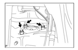
(c) Remove the 3 nuts on the upper side of the rear shock absorber with coil spring.
