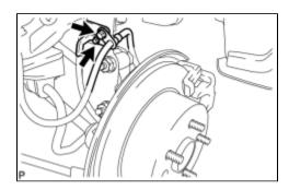
(a) Remove the 2 bolts, and disconnect the rear brake flexible hose and rear speed sensor from the rear shock absorber with coil spring and rear axle carrier.
