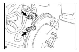
(b) Remove the 2 nuts and 2 bolts on the lower side of the rear shock absorber with coil spring.
