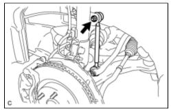
(a) Install the front stabilizer link assembly with the nut.
