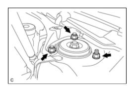
(b) Slowly jack up the vehicle using a wooden block and install the front shock absorber with coil spring (upper side) to the vehicle.
