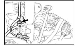
(e) Install the front flexible hose and front speed sensor wire harness with the bolt.
