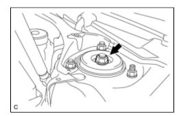
(f) Fully tighten the lock nut.
