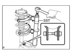
(a) Using SST, compress the front coil spring.
