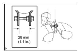
(a) As shown in the illustration, secure the front shock absorber with coil spring in a vise using aluminum plates by clamping onto a double nutted bolt affixed to the bracket at the bottom of the absorber.
