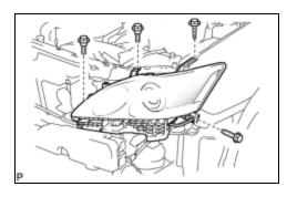
(b) Install the headlight assembly with the 3 bolts and screw.
