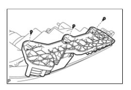
(a) Install the front bumper side support with the 3 screws.
