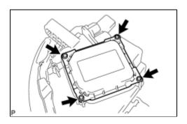
(b) Install the headlight control ECU sub-assembly with the 4 screws.
