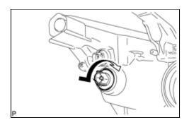
(b) Turn the front turn signal light bulb and front turn signal light socket in the direction indicated by the arrow and install them as a unit.
