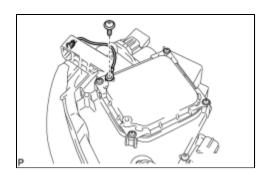
(a) Install the headlight protector with the screw.
