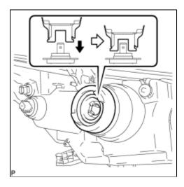
(a) Install the adapter assembly as shown in the illustration.
