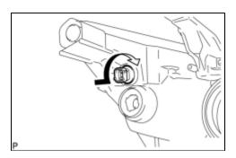
(b) Turn the clearance light bulb and clearance light socket in the direction indicated by the arrow and install them as a unit.
