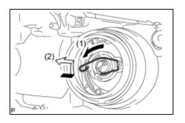
(a) Lock the set spring to install the No. 1 headlight bulb as shown in the illustration.
