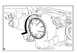
(a) Install the headlight socket cover as shown in the illustration.
