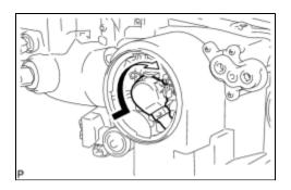
(b) Turn the socket of the light control ECU sub-assembly in the direction indicated by the arrow to connect the socket.
