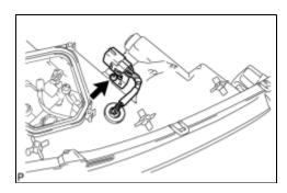
(a) Install the headlight cord with the screw.
