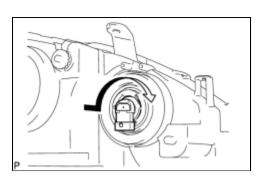
(a) Install the No. 2 headlight bulb as shown in the illustration.
