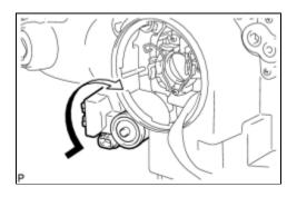
(b) Turn the headlight leveling motor to install it.
