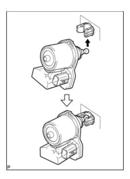
(a) Engage the tip of the headlight leveling motor with the reflector.
