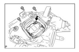
(a) Install the headlight swivel motor with the 3 screws.
