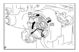
(a) Lock the set spring to install the discharge headlight bulb as shown in the illustration.
