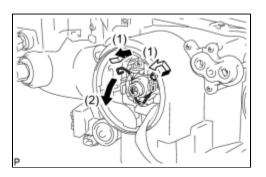
(b) Release the set spring and remove the discharge headlight bulb as shown in the illustration.
