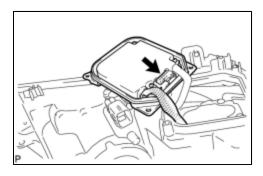
(b) Disconnect the connector and remove the light control ECU sub-assembly.
