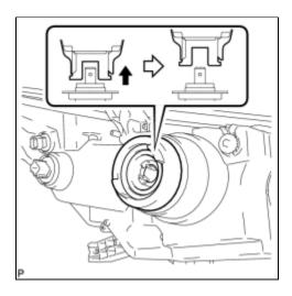
(a) Remove the adapter assembly as shown in the illustration.
