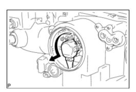
(a) Separate the light control ECU socket as shown in the illustration.
