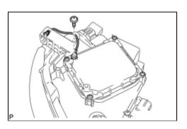
(a) Remove the screw and the headlight protector.
