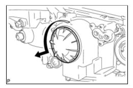
(a) Remove the headlight socket cover as shown in the illustration.
