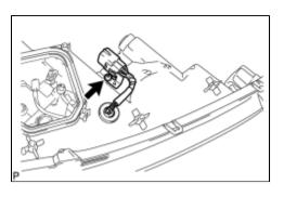
(a) Remove the screw and the headlight cord.
