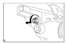
(a) Turn the clearance light bulb and the clearance light socket in the direction indicated by the arrow and remove them as a unit.
