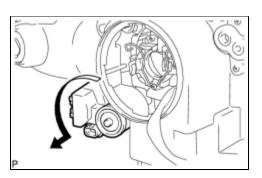
(a) Align the notches of the headlight leveling motor and the housing, and pull out the headlight leveling motor slightly.
