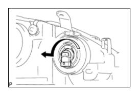
(a) Remove the No. 2 headlight bulb as shown in the illustration.
