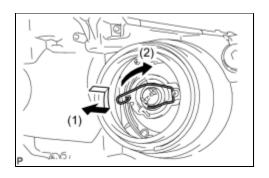
(a) Release the set spring and remove the No. 1 headlight bulb as shown in the illustration.
