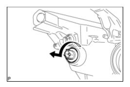
(a) Turn the front turn signal light bulb and the front turn signal light socket in the direction indicated by the arrow and remove them as a unit.
