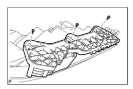
(a) Remove the 3 screws and the front bumper side support.
