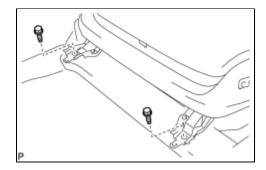
(g) Temporarily install the rear side of the front seat assembly with the 2 bolts.
