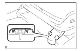
(b) Engage the 2 claws and install the front seat outer track bracket cover.
