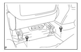
(e) Temporarily install the front side of the front seat assembly with the 2 bolts.
