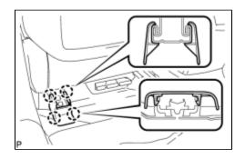
(a) Engage the 4 claws and install the front seat rear outer track cover.
