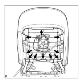
(a) Disengage the hooks.
