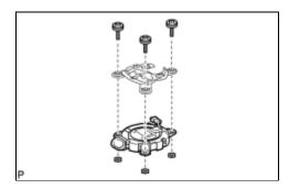
(a) Remove the 3 bolts, 3 nuts, bracket, and seat climate control blower.
