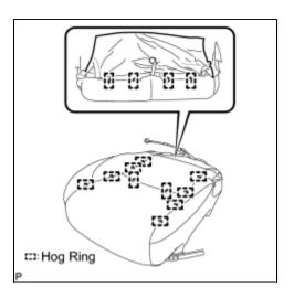
(b) Remove the 14 hog rings and front separate type front seat cushion cover.
