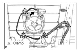
(a) Disconnect the connector and detach the 4 clamps.
