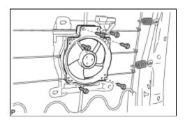
(b) Using a T30 "TORX" socket, remove the 6 "TORX" bolts and remove the seatback climate control blower.
