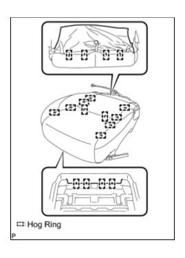
(b) Remove the 18 hog rings and front separate type front seat cushion cover.
