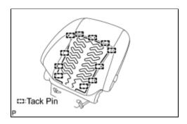
(a) Cut off the tack pins that fasten the seat heater, and then remove the front seatback heater assembly from the separate type front seatback cover.
