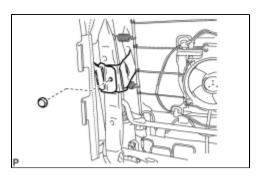
(b) Remove the nut and separate the bracket.
