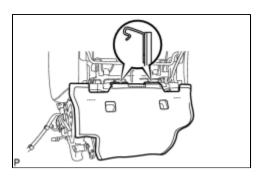
(a) Disengage the hooks and front seatback board cover sub-assembly.
