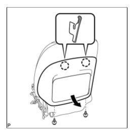
(a) Open the front seatback board cover sub-assembly of the front seatback board sub-assembly. Then remove the 2 screws.
