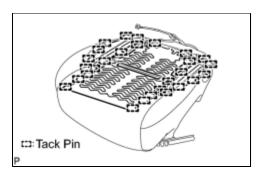
(a) Cut off the tack pins that fasten the seat heater, and then remove the front seat cushion heater from the front separate type seat cushion cover.
