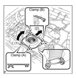
(a) Separate the 2 clamps (A) in the direction indicated by the arrow (1).
