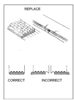
(a) Visually check the V-ribbed belt for excessive wear, frayed cords, etc.
