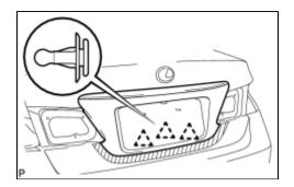
(a) Engage the 3 clips and install the luggage compartment door outside garnish sub-assembly.
