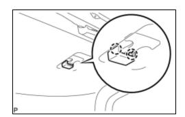
(a) Engage the 2 claws and install the luggage lock control cable plate.
