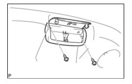
(a) Install the luggage compartment door assist grip with the 2 screws.
