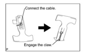
(a) Connect the cable as shown in the illustration, then install the luggage compartment door inside handle.
