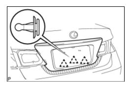
(a) Engage the 3 clips and install the luggage compartment door outside garnish sub-assembly.
