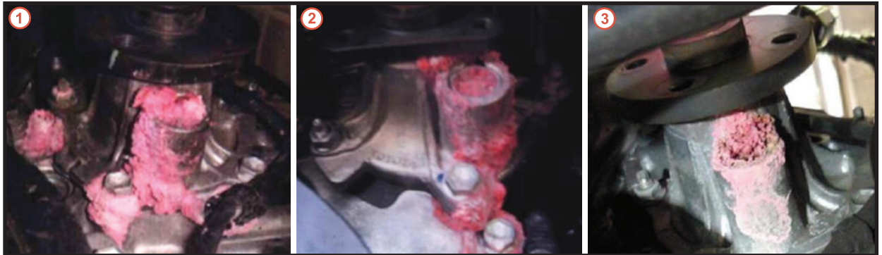
1 Thick coolant deposits present on water pump only 2 Moderate coolant deposits present on water pump only 3 Light coolant deposits present on water pump only
