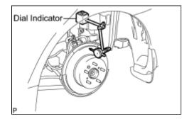
(c) Using a dial indicator, measure the disc runout 10 mm (0.39 in.) away from the outer edge of the rear disc.
