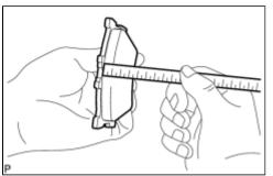
(a) Using a ruler, measure the pad lining thickness.
