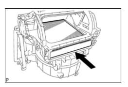
(a) Install the clean air filter as shown in the illustration.
