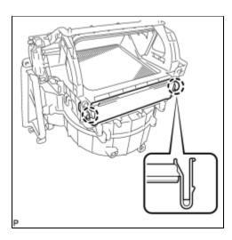
(a) Engage the 2 claws to install the air filter cover plate.
