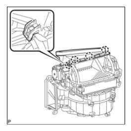
(a) Engage the 4 claws to install the air duct sub-assembly.
