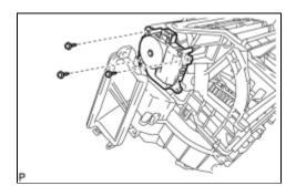
(a) Install the air inlet servo motor with the 3 screws.
