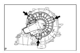
(a) Install the blower with fan motor sub-assembly with the 3 screws.
