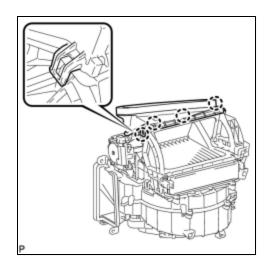
(a) Release the 4 claws and remove the air duct sub-assembly.
