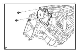
(a) Remove the 3 screws and air inlet servo motor.
