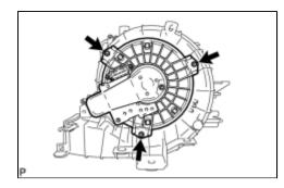
(a) Remove the 3 screws and blower with fan motor sub-assembly.
