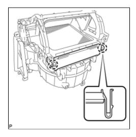
(a) Release the 2 claws and remove the air filter cover plate.
