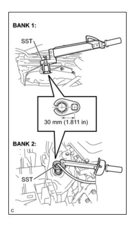
(a) Using SST, install the 2 air fuel ratio sensors to the front pipe assembly.
