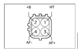
(a) Measure the resistance between terminals 1 (HT) and 2 (+B). Standard resistance:
