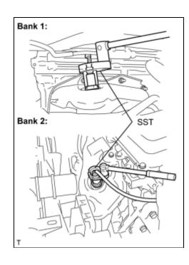
(a) Disconnect the 2 air fuel ratio sensor connectors.
