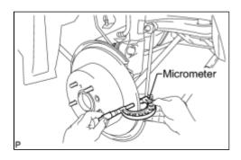
(a) Using a micrometer, measure the disc thickness.
