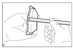
(a) Using a ruler, measure the pad lining thickness.
