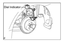
(c) Using a dial indicator, measure the disc runout 10 mm (0.39 in.) away from the outer edge of the rear disc.
