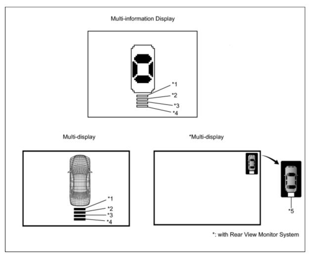
(f) When the ultrasonic sensors (rear clearance sonar) have detected an obstacle, check the display and buzzer sound.
