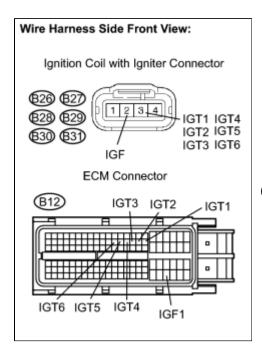
(a) Disconnect the B26, B27, B28, B29, B30 or B31 ignition coil connector.
