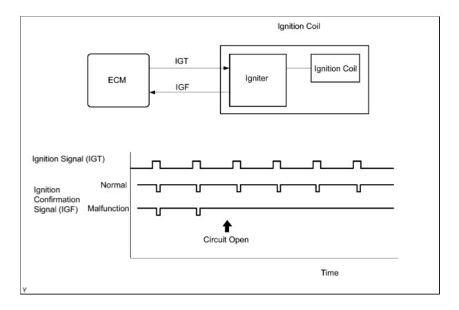
If the ECM does not receive any IGF signals despite transmitting the IGT signal, it interprets this as a fault in the igniter and sets a DTC.
