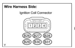
(a) Disconnect the B26, B27, B28, B29, B30 or B31 ignition coil connector.
