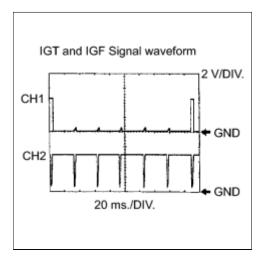
While cranking or idling the engine, check the waveform between terminals IGT (1 to 6) and E1, IGF1 and E1 of the ECM connector.
