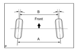
(a) Bounce the vehicle up and down at the corners to stabilize the suspension. Inspect the toe-in.
