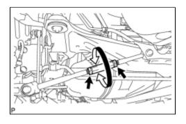
(b) Loosen the lock nuts.
