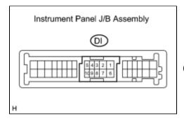
(a) Disconnect the DI instrument panel assembly connector.
