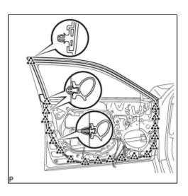
(a) Using a clip remover, disengage the 19 clips and remove the front door weatherstrip.
