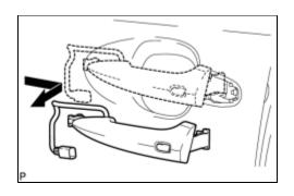
(e) Remove the front door outside handle assembly as shown in the illustration.
