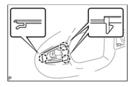
(a) Disengage the 3 claws and remove the front door front outside handle pad.
