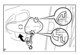
(a) Using an emergency key, disengage the 2 claws and remove the front door outside handle cover.
