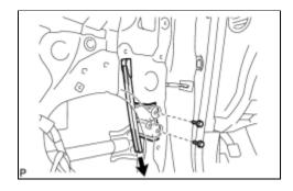
(a) Remove the 2 bolts and the front door front lower frame sub-assembly as shown in the illustration.
