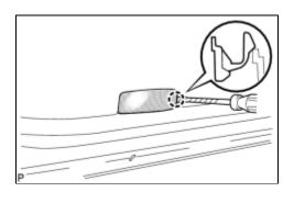
(a) Using a screwdriver with the tip wrapped with protective tape, disengage the claw and remove the courtesy light assembly.
