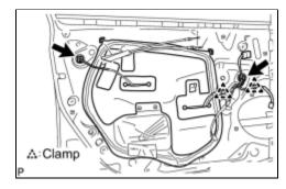
(a) Disconnect each connector and each clamp, and remove the front door service hole cover.
