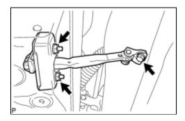
(a) Remove the bolt, 2 nuts, and front door check assembly.
