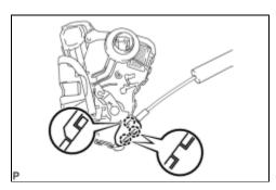
(a) Using a screwdriver, disengage the 3 claws.
