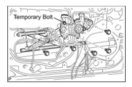
(a) Loosen the temporary bolt.
