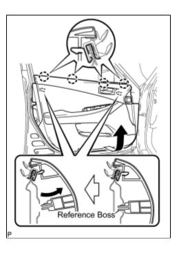
(c) Pull up the front door trim board in the direction indicated by the arrow.
