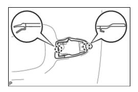
(a) Disengage the 2 claws and remove the front door rear outside handle pad.
