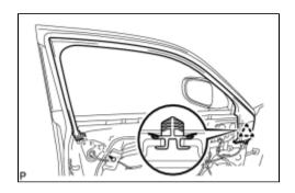
(a) Using a clip remover, remove the clip.
