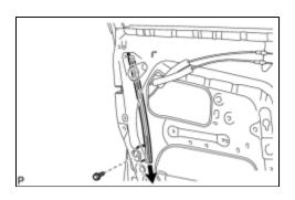
(a) Remove the bolt and the front door rear lower frame sub-assembly as shown in the illustration.
