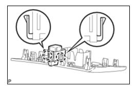
(a) Disengage the 2 claws and remove the door control switch assembly.
