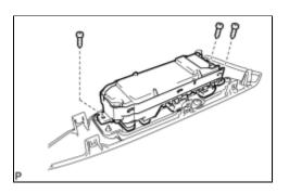
(a) Remove the 3 screws and the power window regulator master switch assembly.
