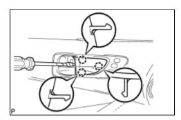
(a) Using a screwdriver with the tip wrapped with protective tape, disengage the 3 claws, and remove the front door inside handle bezel plug.
