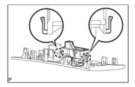
(a) Disengage the 2 claws and remove the power window regulator switch assembly.
