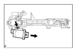
(a) Remove the screw and door electrical key oscillator.
