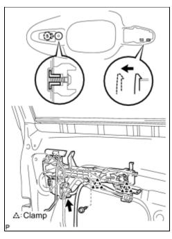
(a) Using a "TORX" socket wrench (T30), loosen the screw.
