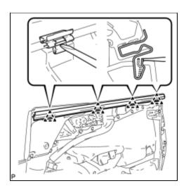
(a) Disengage the 4 clips as shown in the illustration and remove the front door inner glass weatherstrip from the front door trim board.
