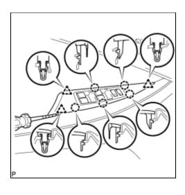
(a) Using a screwdriver with the tip wrapped with protective tape, disengage the 5 claws and 3 clips, and remove the front door armrest base panel assembly.
