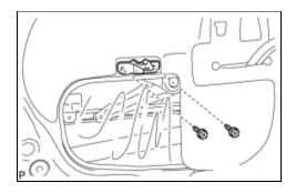
(a) Remove the 2 screws and the front No. 1 door trim bracket.
