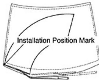
Alignment of the right wiper blade front end at the rest position.
