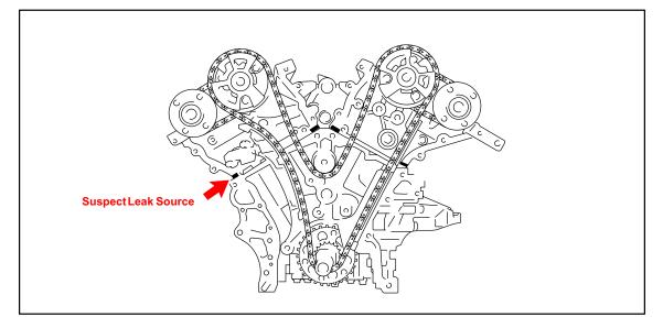
3. Remove and reseal the timing cover if confirmed leaking.
