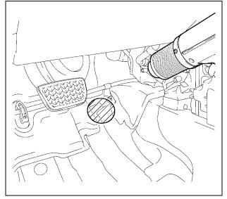
2. Using a hair dryer or low temperature heat gun, warm up the sound deadening material until it becomes soft.
