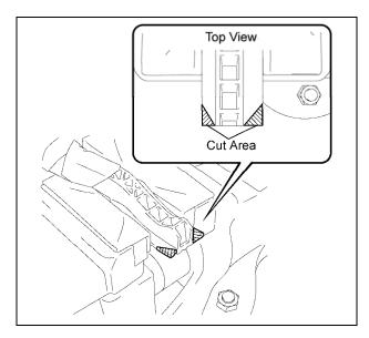
b) Using a reciprocating saw, cut the corners of the pedal.
