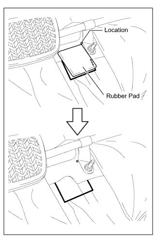
1. Temporarily place the rubber pad on the floor panel as shown, and outline the pad on the sound deadening material with a ball point pen.
