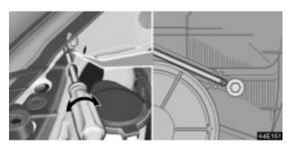
2. Turn the vertical movement adjusting bolt 2 the same number of turns and in the same direction as step 1 using a Phillips—head screwdriver.
