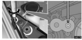
1. Turn the vertical movement adjusting bolt 1 in either direction using a Phillips-head screwdriver. At this time, keep the turning direction and number of turns in mind.
