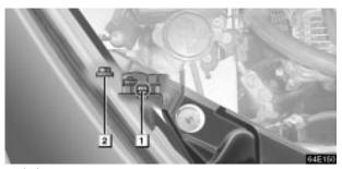
▶ 1 Vertical movement adjusting bolt 1 2 Vertical movement adjusting bolt 2
