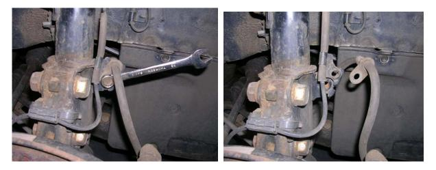
(b) Remove the bolt and disconnect the front flexible hose and front speed sensor wire harness from the front shock absorber with coil spring.
