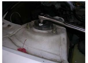
(a) Loosen the lock nut of the front shock absorber with coil spring.
