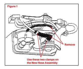
Install the New Hose Assembly as shown in Figure 2. Reuse the Hose Clamps removed in Step 2 on the large hose as indicated.
